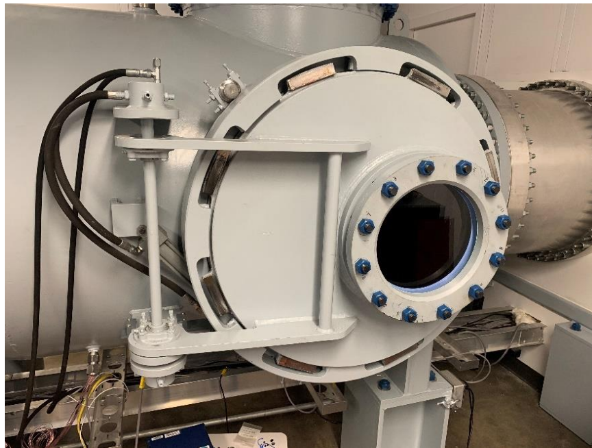
Figure 9. Autoclave door with optical access
